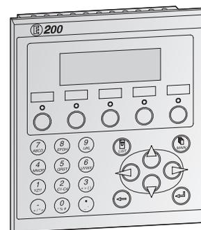
The **E200** terminal offers 5 programmable function keys with freely definable labels and alternating function assignment. LEDs indicate the process status. Recipes, passwords, texts, alarms and changes can be entered via input keys. The E200 offers an LCD display with four rows and 20 characters each. It poses one RS232C port and a RS422 port, which can be connected to either two PLCs or a PLC and a printer, bar code reader and other RS232 devices.
