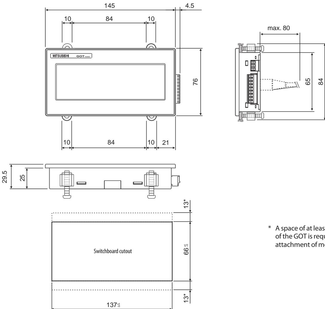
\* A space of at least 13 mm at the long side of the GOT is required to allow for the attachment of mounting fixtures.
