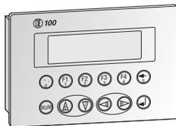
The **E100** has 4 programmable function keys with freely definable labels and alternating function assignment. Recipes, passwords and changes can be entered via input keys. The unit has an LCD display with two rows and 20 characters each. It has one RS232C port and a RS422 port, which can be connected to either two PLCs or a PLC and a printer, bar code reader and other RS232 devices.
