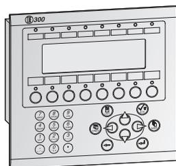
The **E300** has a key-oriented user interface with programmable function keys. The graphical screen can display symbols, alarms, graphs and texts in a variety of sizes. Recipes, passwords, texts, alarms, and changes can be entered via input keys.
