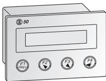
The **E50** is a key-oriented HMI unit with four function keys and an LCD display with two rows and 16 characters each. It can display up to 50 text blocks, which can be paged with the function keys. Values can be edited directly with the unit's keyboard. The RS232C and RS422 ports are both integrated in a 25-pin connector.
