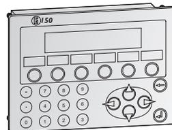
The **E150** unit features 6 programmable function keys with definable labels and numerical keypad. Recipes, passwords and editing changes can all be entered and edited directly with the units keyboard. The unit offers an LCD display with two rows and 20 characters each. It has one RS232C port and a RS422 port, which can be connected to either two PLCs or a PLC and a printer, bar code reader and other RS232 devices.
